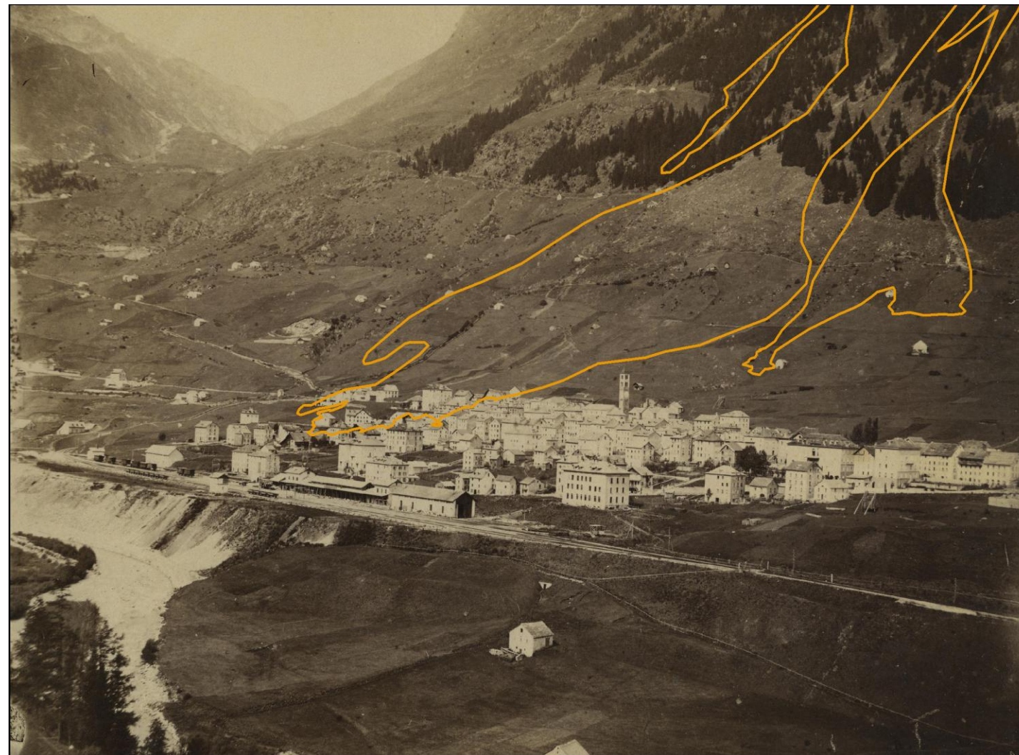
Projection of the rockslide perimeter on an oblique terrestrial image of the area prior to the event.
